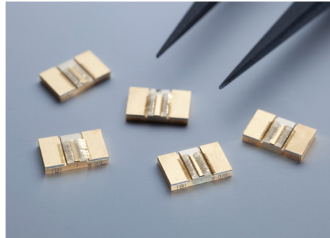
Fig. 1. FBH standard test format: broad area lasers ( L = 4 \text{ mm} , w = 90 \mu\text{m} ) soldered with AuSn onto CuW screening submounts for cw testing at T_{\text{HS}} = 25^\circ\text{C} .
