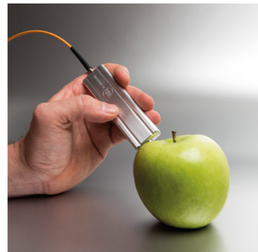
Fig. 2. Realized SERDS probe for in situ Raman investigations.
